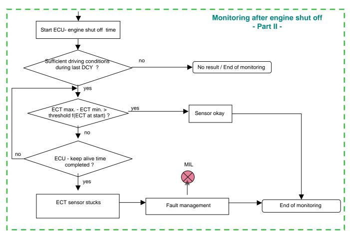
Engine Coolant Temperature Sensor Out of Range Check (P0118 / P0117)
