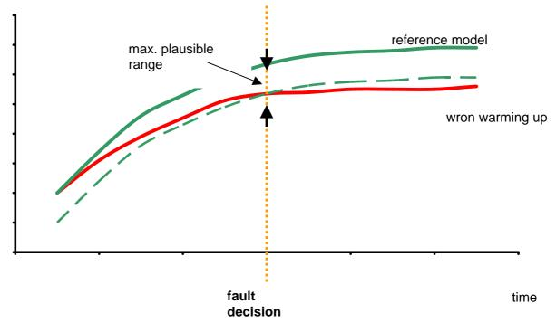
Flow Chart Coolant Temperature Sensor Rationality (P3081)
