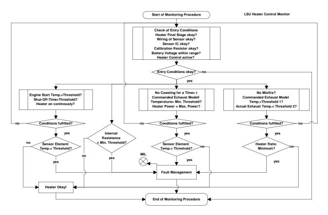
Flow Chart: LSF1/LSF2, Oxygen Sensors downstream catalyst
