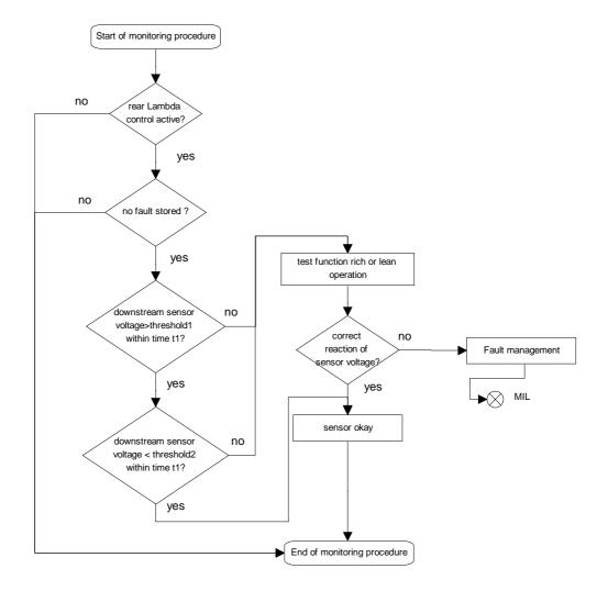
Flow chart: Oscillation Monitoring (LSF1/2 O2 Sensor Downstream Catalyst)
