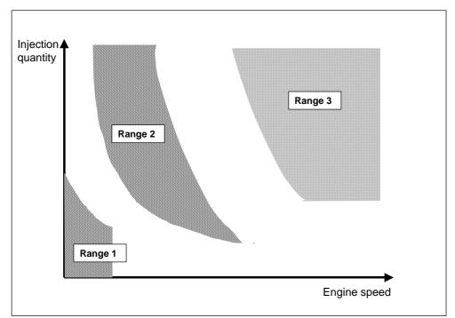
Lambda deviations in **range 1** are compensated by an additive correction value multiplied by an engine speed term. This creates an additive correction per time unit.
