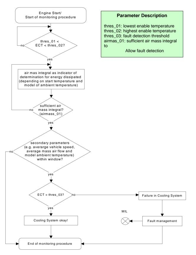
Engine Coolant Temp. Sensor Rationality (P3081)
