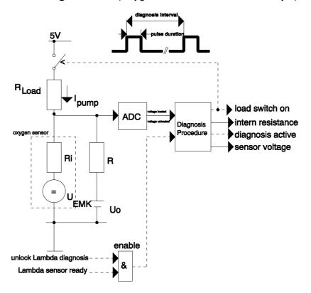
Monitoring Structure (Oxygen Sensor Downstream Catalyst)
